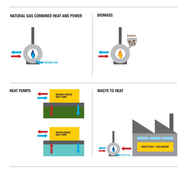
Of these heat generating plants, the natural gas, biomass and waste heat options can also produce electricity and this is known as Combined Heat and Power (CHP). Heat pump systems do not produce enough heat to enable them to create electricity and are therefore more limited in scope, although they are used in small scale domestic heat networks such as Devon & Cornwall Housing Association's housing scheme in Penzance, Cornwall.
