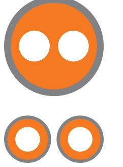
Twin pipe: both the feed and return pipes are contained in one insulated casing. Twin pipe is currently always a polymer (plastic) pipe and there are two types of insulation that can be chosen, PU foam (polyurethane) and PEX foam (crosslinked polyethylene).
